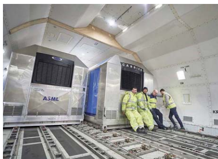
HEADED EAST: A portion of an ASML NXE:3350B EUV scanner is loaded onto a 747-400 extended-range freighter at the Amsterdam Airport Schiphol in the Netherlands, for shipment to a customer. The scanner is split into nine parts (some larger than others) for shipping.
